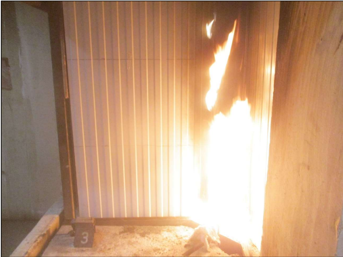
PHOTO Nº9: Sample 3 – Flame attack approx. 10 minutes after the start of the test.
