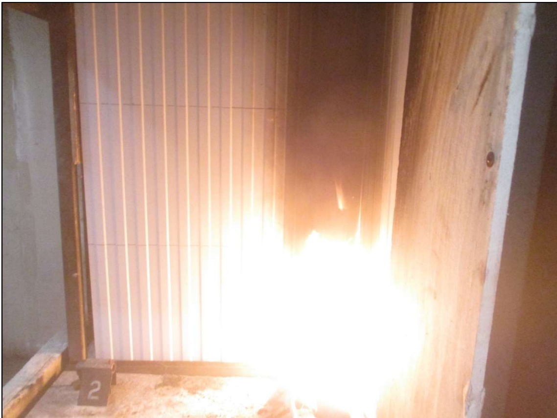
PHOTO Nº7: Sample no. 2 - Flame attack approx. 10 minutes after the start of the test.
