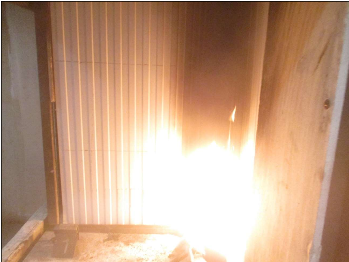
PHOTO Nº5: Sample 1 – Flame attack approx. 10 minutes after the start of the test.
