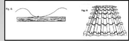
Caution: Special attention should be shown to the line of attachment where one sheet overlaps the previous one (Fig, I) A good fixation secures an optimal fit to each other
